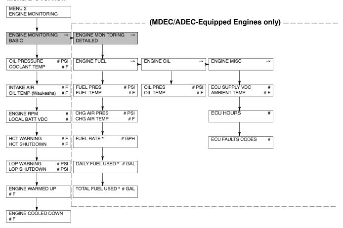
\* While these menu displays do appear on the 550 controller, the engine ECM is not currently set up to provide this data.
